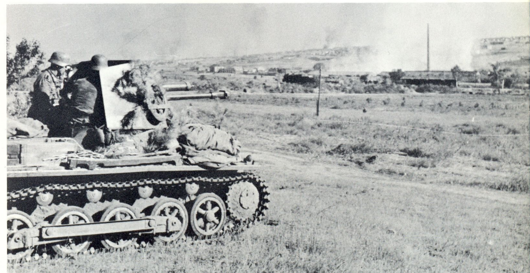
The Panzerjäger I was constructed by removing the machine-gun armed turret of the Panzerkampfwagen I and adding light armor plating over the top decking and around the Czech-built 47mm anti-tank gun to protect the crew. The gun was effective at short and medium ranges against most armor, but not the larger Soviet and British tanks.
