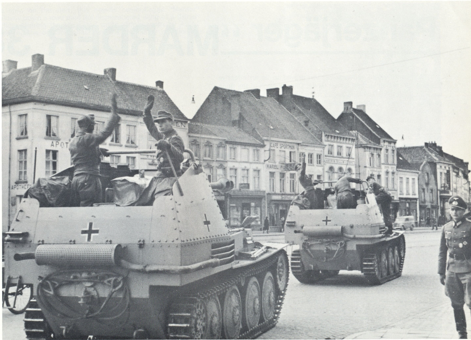
Fresh crews and new vehicles. These Sd. Kfz. 138 " Marder 38's " move through a small town on their way to the front. Note the exhaust pipes and mufflers at the rear of the vehicles and the exhaust leads that extend from the middle of the chassis backwards, indicating that the engines are mounted in front of the gun positions.
