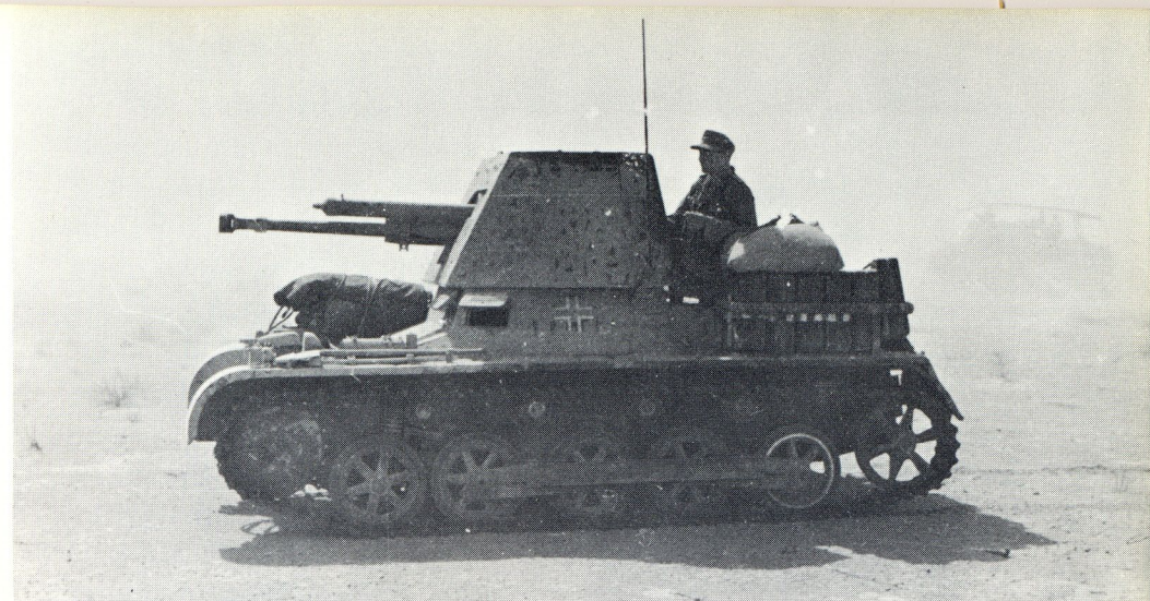
The Panzerjäger I , Germany's first WWII self-propelled anti-tank vehicle, was built on the chassis of the Panzerkampfwagen I , Ausführung B, a German tank that was developed during the Spanish Civil War and also served in Poland and France.
