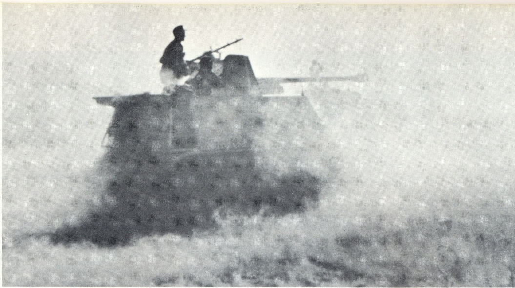
A Marder III at work on the Eastern Front. The gunner loads another big round as the smoke and dust from the previous firing settles around the vehicles. Notice that the vehicle has been fitted with an MG34 machine gun, mounted on the side of the gun shield.
